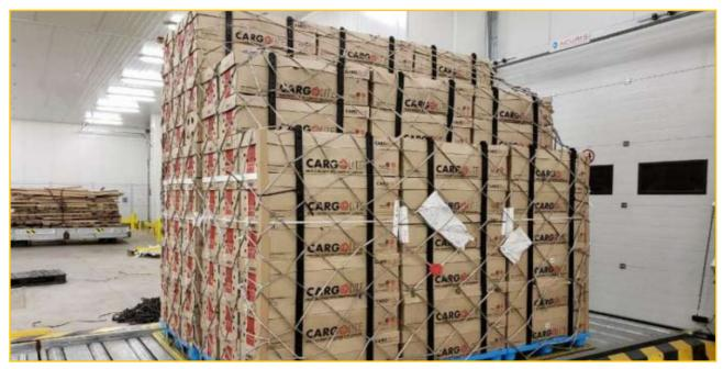
Completed air pallets with cartons neatly arranged in layers. The black frames form a supporting system that diverts the load from the carton walls to the frames.
