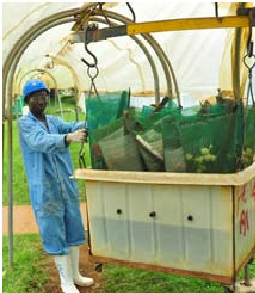
The environmental friendly railing system that transports flowers from greenhouses to packhouses at Redlands Roses
